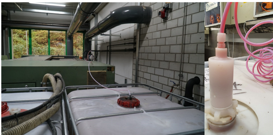
Figure 15: Exemplary pictures provided by DUs displaying the concentration adjustment with liquid CrO 3 using a standard connection (left) and K.Walter's Quick Connect system (right; only removal head and hose shown)
