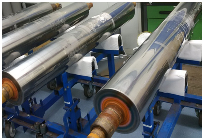
Figure 9: Chrome plated gravure cylinder.
