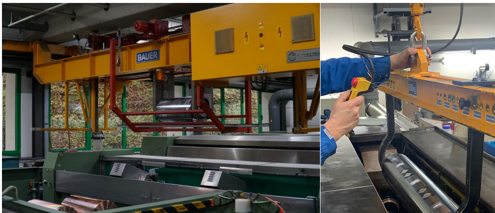
Figure 12: Exemplary pictures from DU sites of the automatic (left) and manual (right) loading and unloading process of the electroplating unit
