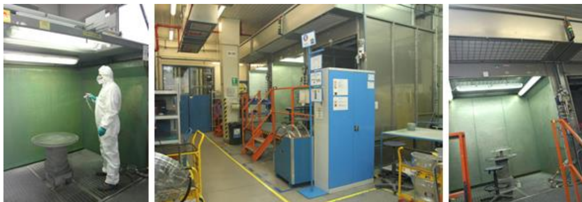
Fig. 4: Manual painting application of several coating layers in open paint booth.
