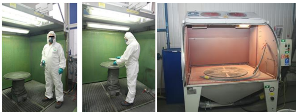
Fig. 3: Preparation of the painting-coating process: Masking and sandblasting.
